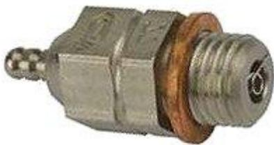
Where a petrol engine uses a spark plug to ignite the fuel/air mixture within the compression chamber, so an rc model airplane glow engine uses a small glow plug.
