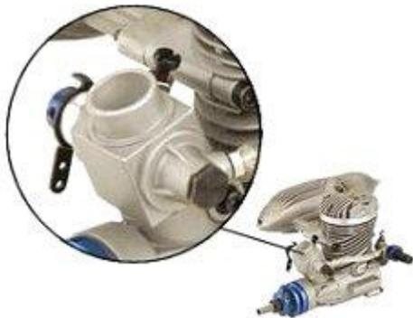
Model airplane engines have a very simple carburettor, generally speaking. It's typically located on the top front of the engine crankcase, although some newer engines have the carb located at the rear for safer adjusting (to keep fingers well clear of the propeller).
