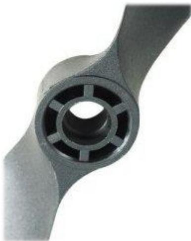
One is to balance the **hub** of the prop. This method is better for larger props (with bigger hubs) rather than your average park-flyer size propeller with hubs that are really too small to try and balance easily.
