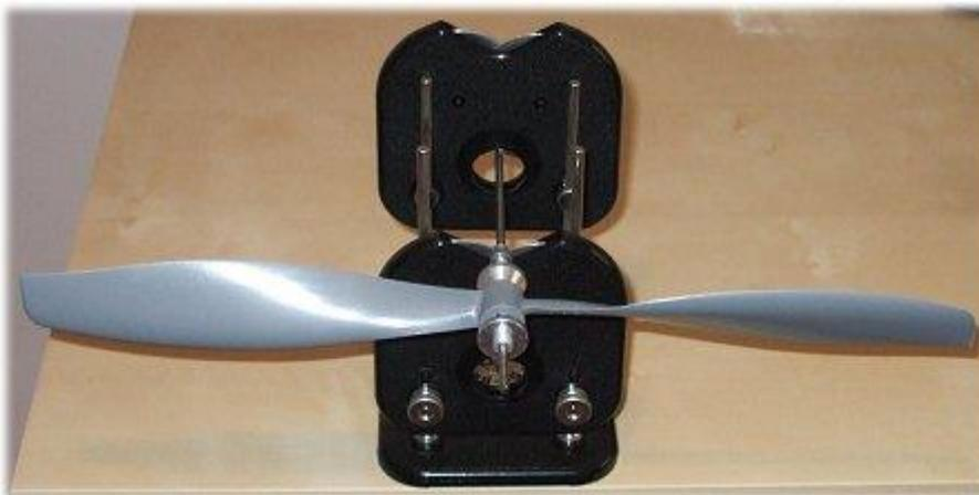
Above: A correctly balanced prop will come to rest, at *any* position, without tipping one way or the other. Don't look for just a 3 o'clock – 9 o'clock position, as shown above.
