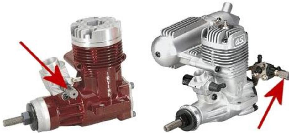
Above: the location of the all important needle valve. Modern engines may have the valve at the rear (right), but many engines have the needle on the carburettor (left).
