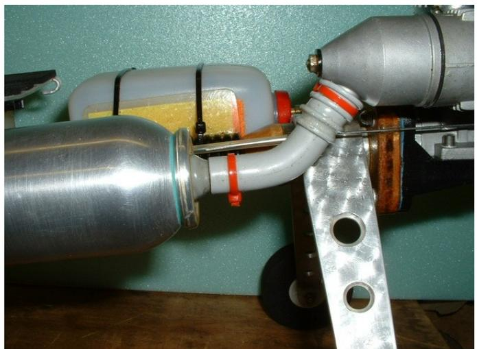
The muffler can be mounted to the airframe using tie-wraps / elastic bands / fuel tube & self tappers or wire.
